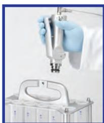
Squeeze trigger and press the thumb button until it locks.
