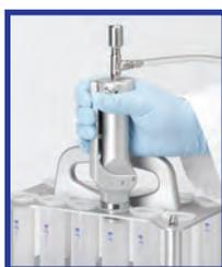
In this position, a constant pressure is maintained in the column without holding the trigger.
