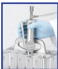
Release trigger. O-ring now forms a gas tight seal within the column.
