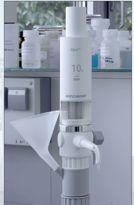
Adapter with NS 12/21 filling tube for funnel. The adapter with standard ground 12/21 filling tube enables problem-free filling of medium through a funnel - without unscrewing the basic unit.
