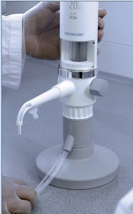
Base support instead of bottle attachment. The base support enables suctioning of the medium directly from a separate storage container using a hose.
