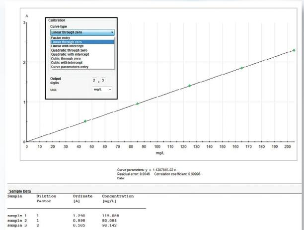
Quantitative analysis gives you flexibility to fit multiple curve types or enter a factor. Customize your data display precision and result unit. Result reports include the calibration graph, curve fit, standard solution data and experimental results.
