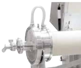
Water-cooled vacuum flange (gas supply system 2)
