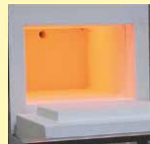
Muffle heated from four sides
