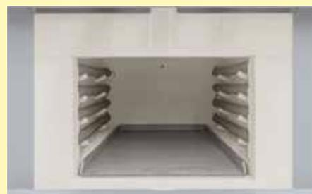
Deep furnace chamber with three-sides heating
