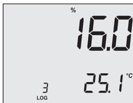
Pressing the arrow keys, the instrument will display the same parameter but for a different record:
