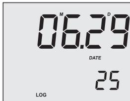
The instrument displays then the amount of free log space for about one second and returns to normal measurement mode (e.g. 18 records free).
